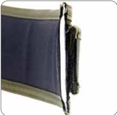
The inner belt is constructed with friction fabric on the inside, then foam, then hard plastic, then fabric and finally hook Velcro. The outer belt is made with loop Velcro on the inside, then hard plastic, and webbing on the outside.
